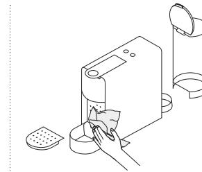
**② Dry with a fresh and clean towel, cloth or paper and reassemble all parts. Clean the coffee outlet and inside the machine regularly with a damp cloth.**
