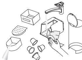
**① Empty the drip tray, the drip base and the capsule container every day. Also remove the water tank with its lid and clean them all with odorless detergent and rinse with warm / hot water.**
